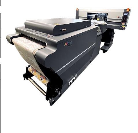
The applicator should be vented outside but can be vented into an air purifier capable of handling up to 285 degrees Fahrenheit. The applicator has a 2" hose ported out from the bottom.
